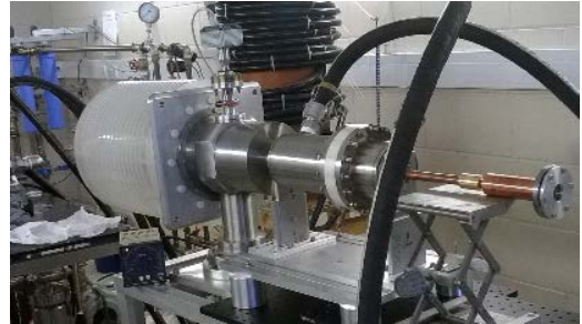
Figure 1 Photograph of 2D PSL high power mm-wave source showing the Blumlein pulser, diode, output horn and window.
