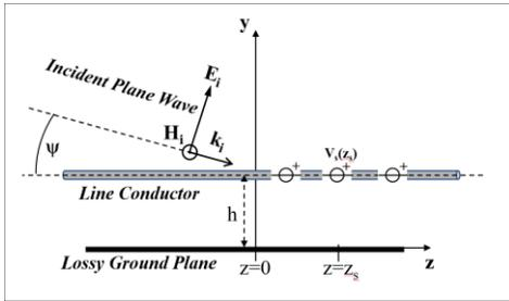
Figure 1. Incident wave on line above ground
