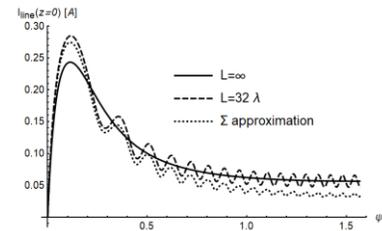
Figure 2. Line current amplitude vs. incidence angle  $\psi$
